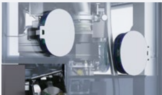
The double rotary press is dust-tight as standard and also available with a containment package.
